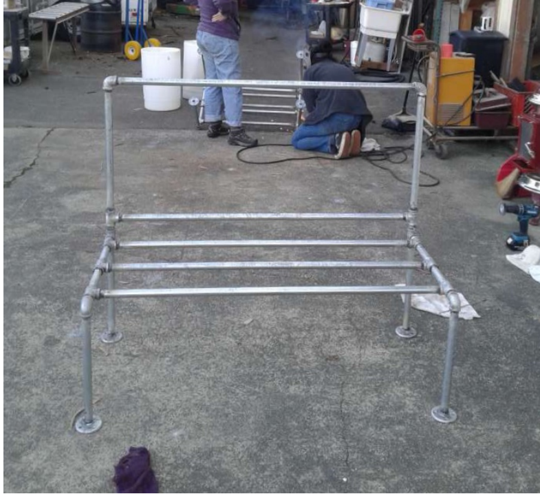
Figure 54: The frame of the larger of the two benches assembled and welded.
