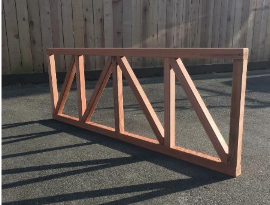
Figure 5.4.3.1: The completed Truss Section.
