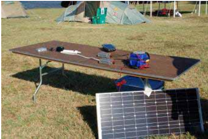
80 W Solar Panel Charging AA Batteries
