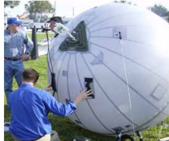
ShelterBox supports 10 people GATR Inflatable SATCOM Dish provides bandwidth
