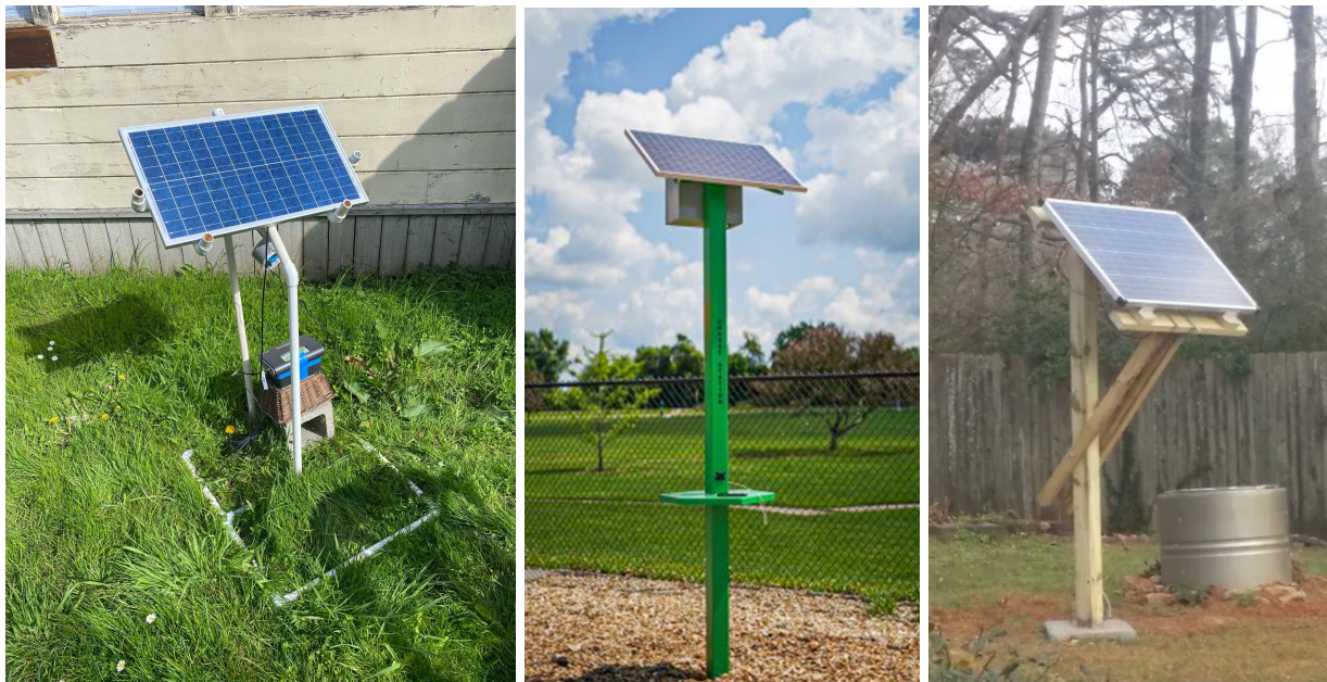
Figure 3. The team's solar PVC prototype on the left, the proposed metal system design from WillyGoat.com, and the proposed wood system design by Born to Build from the Autodesk Instructables website.
