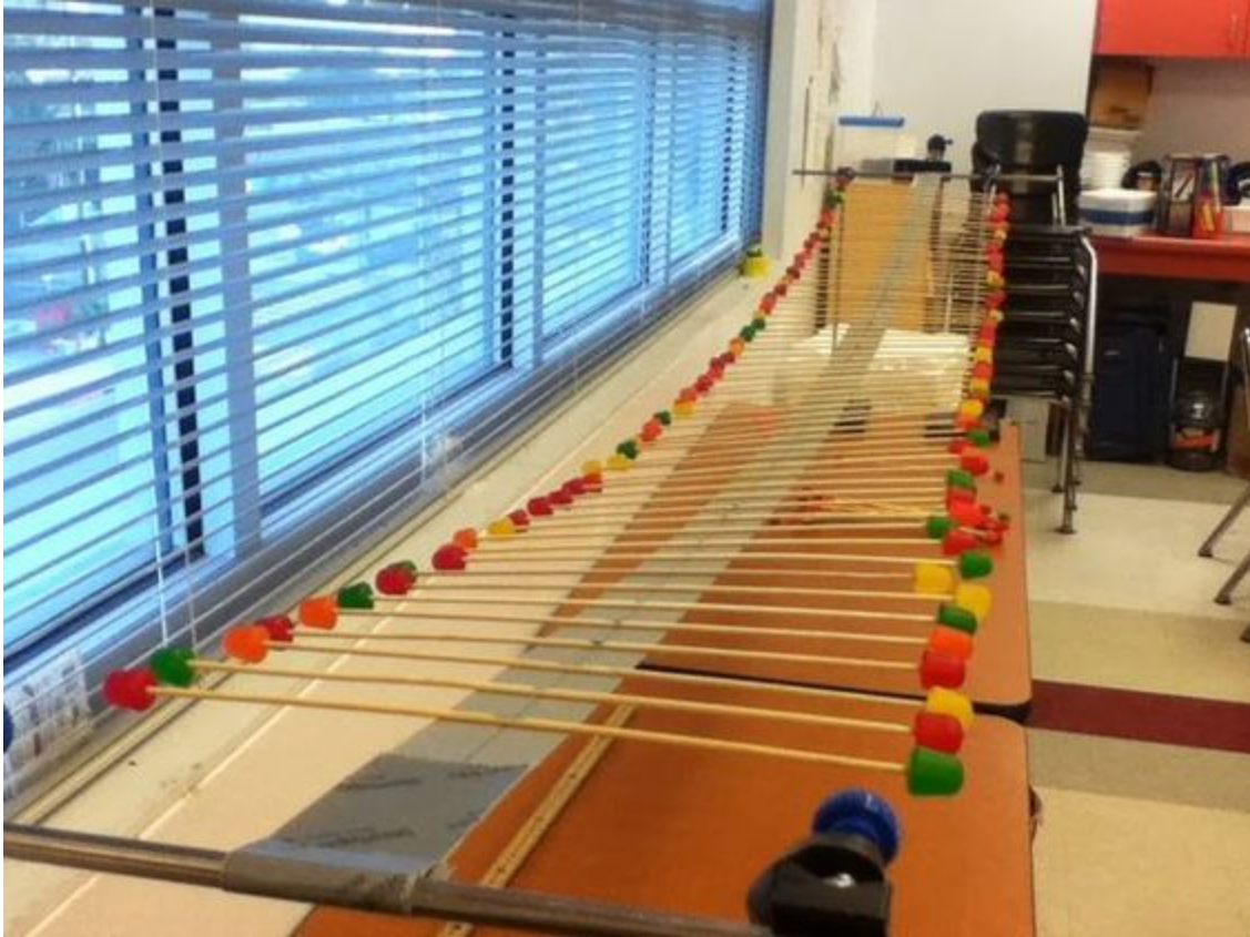
Figure 3-6: In a duct tape Pendulum wave machine, the pendulums can be removed to show that waves move at different speeds in different mediums ( Nakaya et al. ).
