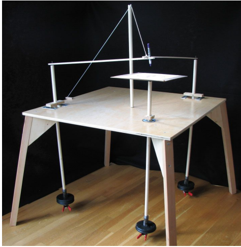
Figure 2-4 A standard harmonograph with two pendulums that swing to move the pen back and forth (Sims, 2009).
