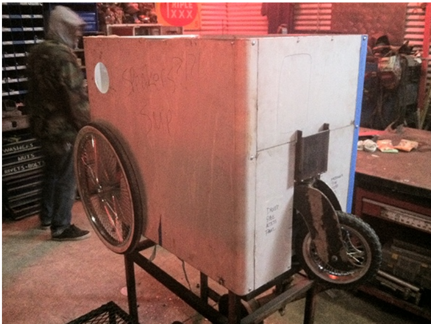
Figure 2-4 Paleta cart with insulation and outer walls
