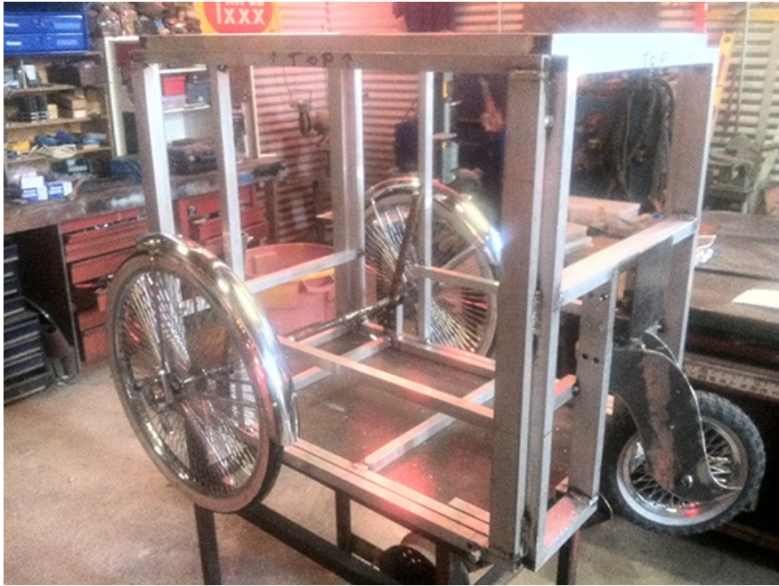
Figure 2-3 Paleta cart frame with real wheels
