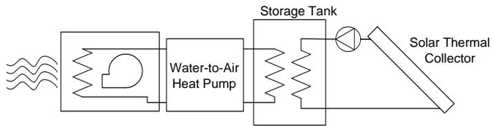
Figure 4. Simplified schematic of SAHP with water tank storage
