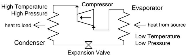
Figure 1. Heat pump shown in heating mode.
