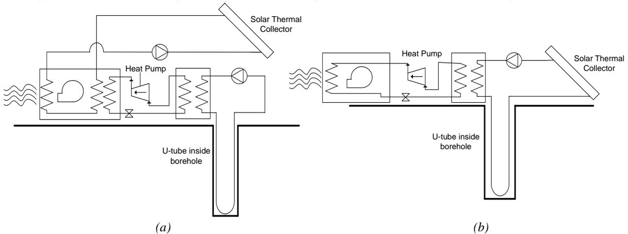
Figure 6. Simplified schematic of a solar assisted ground-source heat pump system (a. parallel, b. series) shown here for air space heating
