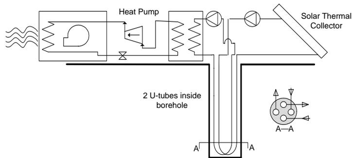
Figure 7. Simplified schematic of the 2 U-tube configuration proposed by Bernier and Shirazi (2007)
