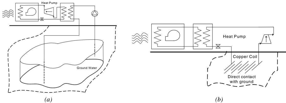
Figure 3. Simplified schematic of a ground-source heat pump system (a. open loop, b. direct exchange) shown here for air space heating
