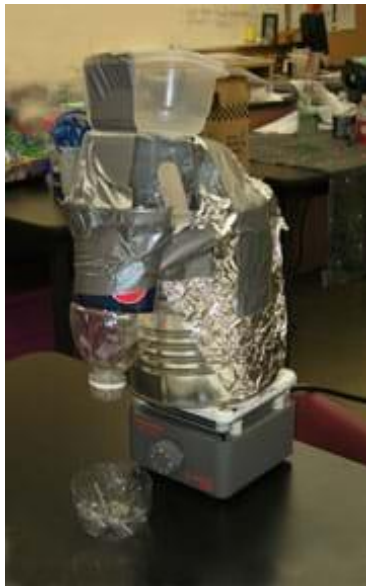
Figure 2-3: An experimental thermal process desalination device. (Carleigh Samson 2009)
