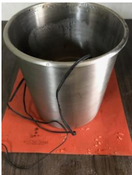
Figure 5-7: Prototype of the heating element. Photo credit: Chris Koier.
