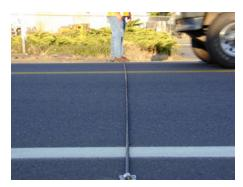
Always keep some tension on the hose with your foot while working with it on the near side so a passing vehicle doesn't pick it up.
