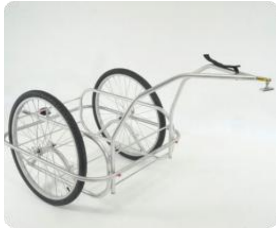
Figure 3-5 A Platform style trailer that has a deck that is below the axle centerline for lower center of gravity and increased stability (Cycle Tote 2013).
