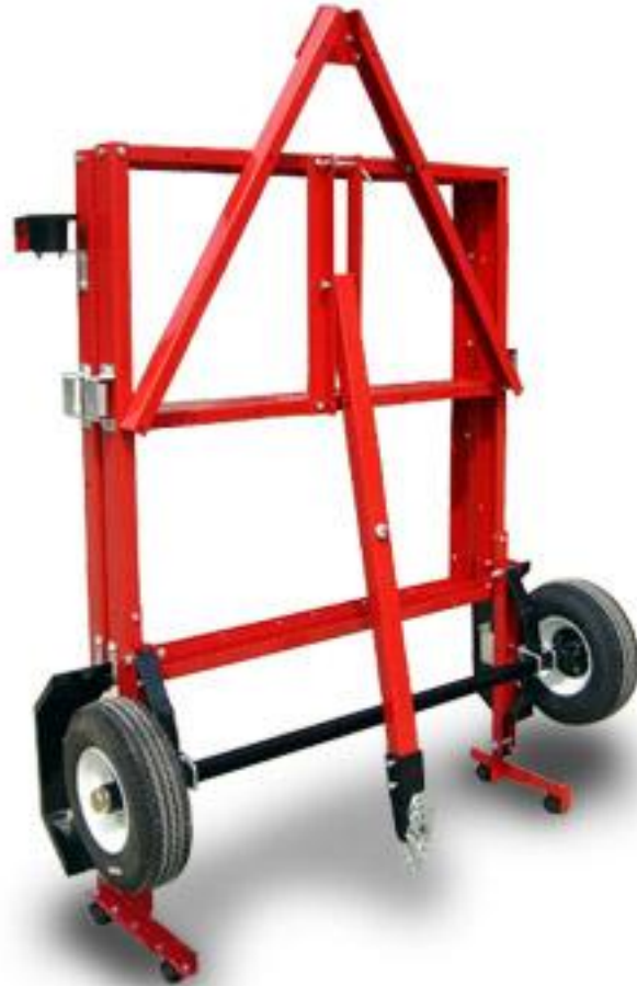
Figure 4-4: An automobile utility trailer stored on hind end casters (Red Trailers 2013).
