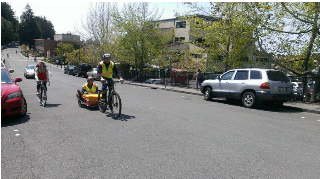
Figure 5-8: Uphill towing test with 155 lb cargo (Kennedy 2013).
