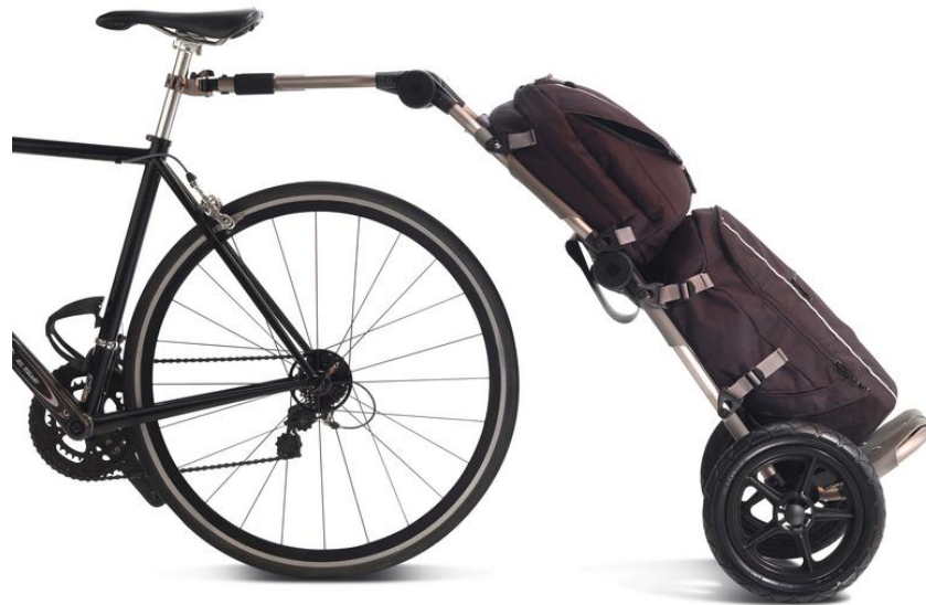
Figure 3-6 An angle style frame trailer (Burley 2013).
