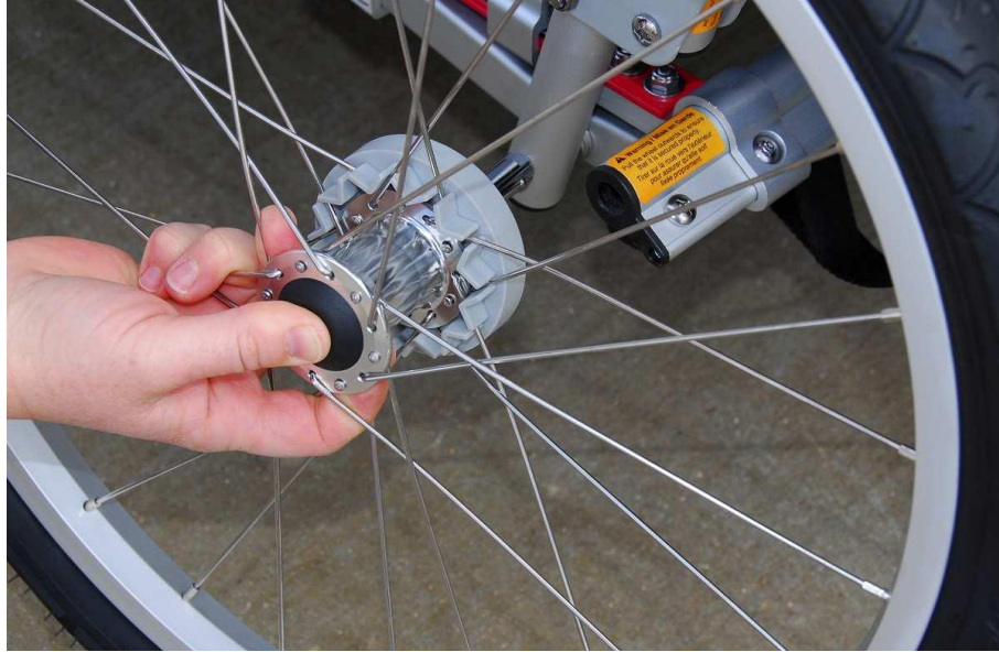
Figure 4-3: Removable bicycle style wheels on a bike trailer (Speed Pedal 2010).
