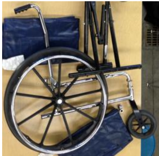
Figure 5-2: Our wheelchair wheels and stub axles (DeMaranville 2013).
