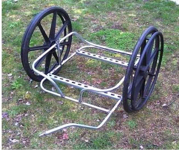
Figure 4-8: A Conduit frame with wheel chair wheels (Bike Shop Hub 2010).
