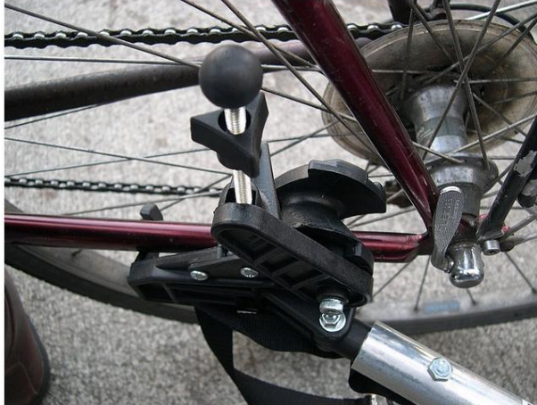
Figure 3-10 An elastomer style hitch that clamps to the rear triangle of the towing bike (Kellogg 2006).
