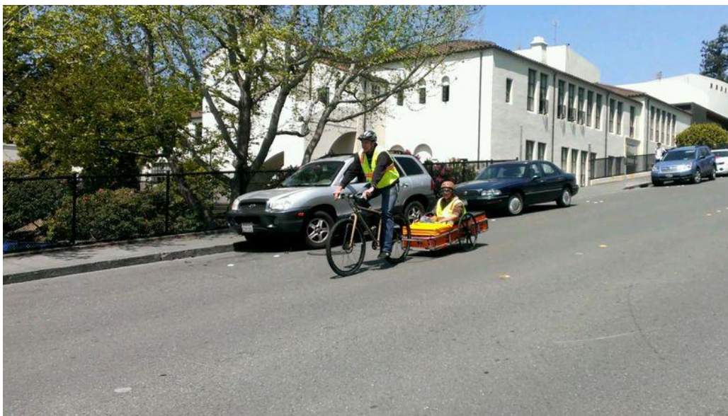
Figure 5-7: Downhill braking test with 155 lb cargo (Kennedy 2013).
