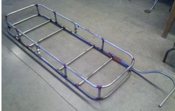
Figure 5-3: 3/4" Electrical conduit frame (Adams 2013).
