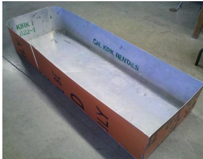
Figure 5-4: Tub-o-Metal formed from a highway sign (Adams 2013).
