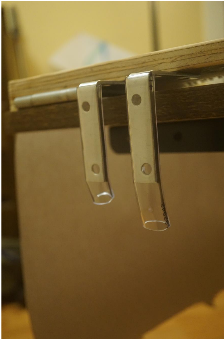
Figure 5-5: L-Bracket System implemented on backside of the Inspirograph (Photo by Aren Page)
