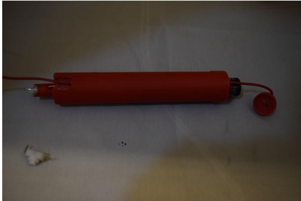
Insert the LED case into the otoscope body
