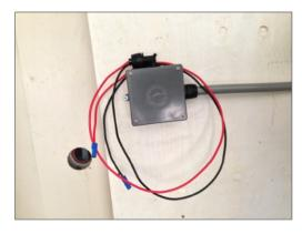
**Step 5 :** Plug BLUE connectors from step up convertor to BLUE connectors MEOW's battery bank.
