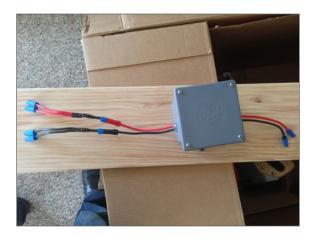
**Step 4 :** Plug both bikes into the step up converter **RED** wires to **RED** wires and **BLACK** wires to **BLACK** wires
