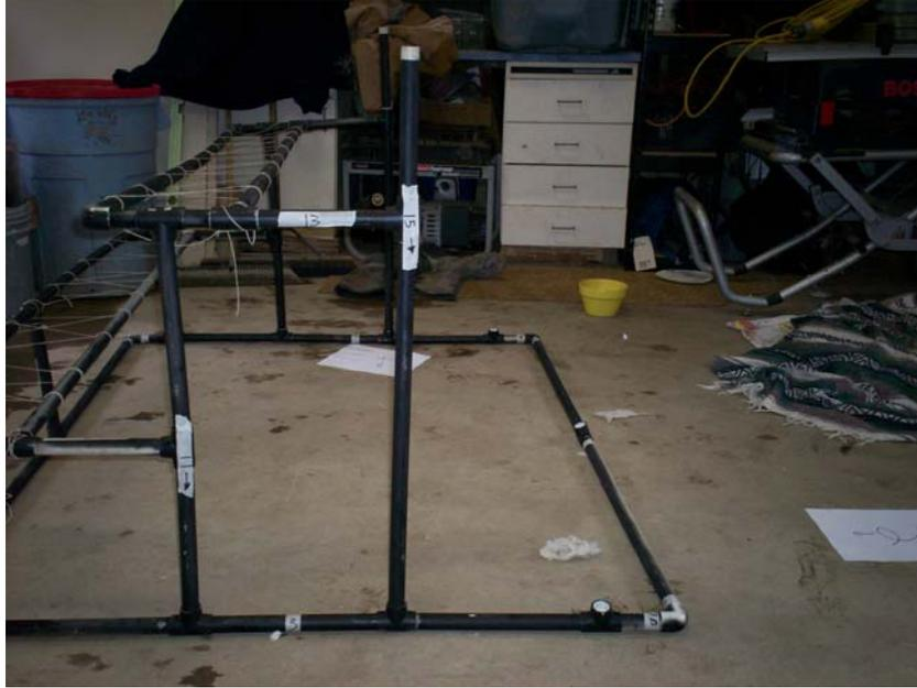
Figure 35: Pipe sections 12,13,14, and 15 assembled (Note Directional Arrows)
