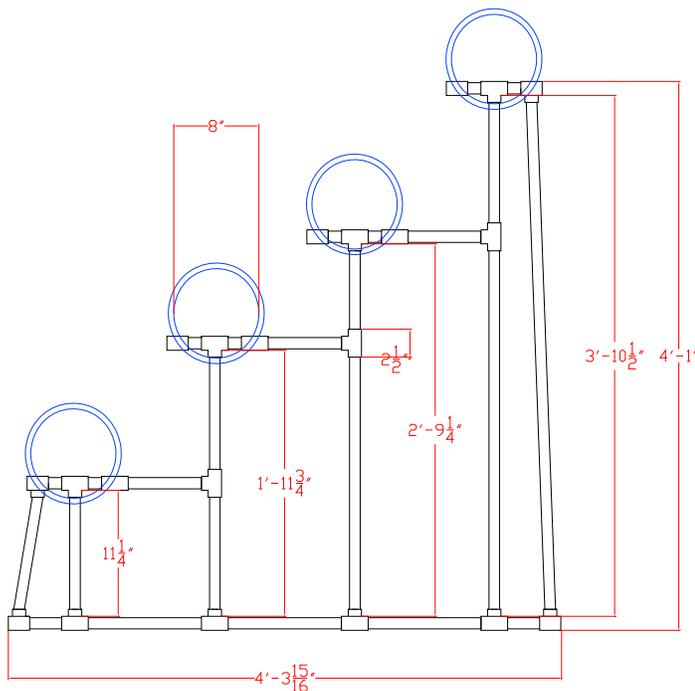
Figure 13, AutoCAD Side view of Drip Hydroponic System
